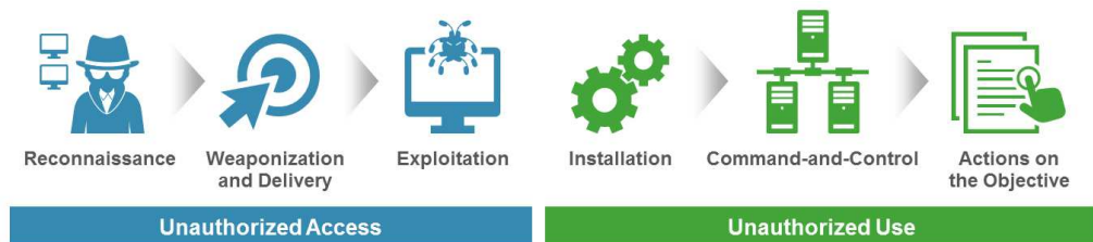
Figure 2: The Palo Alto Networks Attack Kill Chain Model
