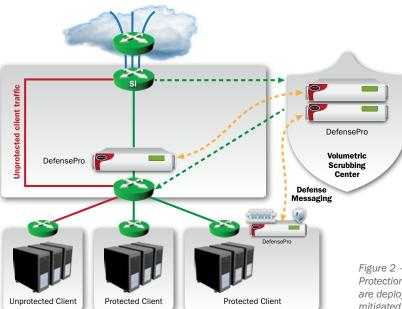
Figure 1 – Always- on deployment of AMS components: Each protected customer has a dedicated security policy on the shared devices; volumetric attacks are mitigated in the scrubbing center.
