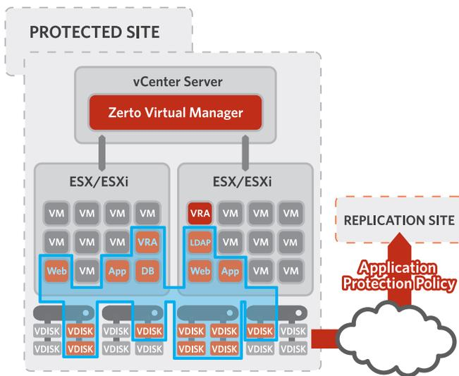
Figure 3 - Application Protection: Virtual Protection
