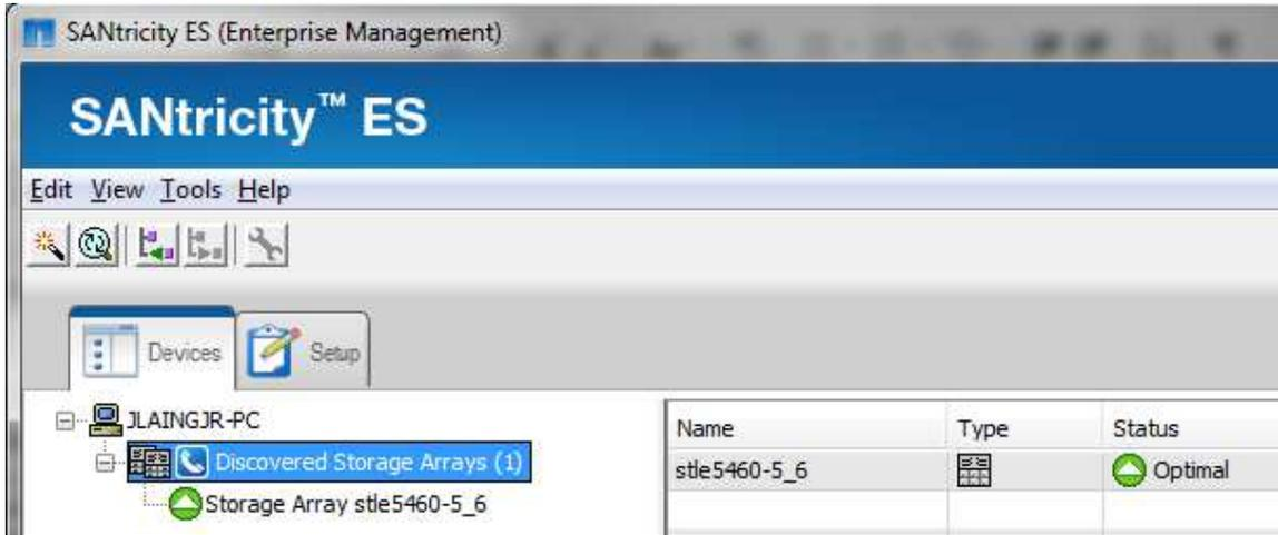
5. Double-click the array to be managed to open the Array Management window (AMW). Use the Summary and Hardware tabs to verify that the status of the array is Optimal (green) and that all expected drives and controllers are seen. If it is not Optimal and if not all the expected drives are shown, rectify these conditions before proceeding to the next step. (The details in the screenshot shown here may not exactly match your test environment.) The AMW is shown here.
