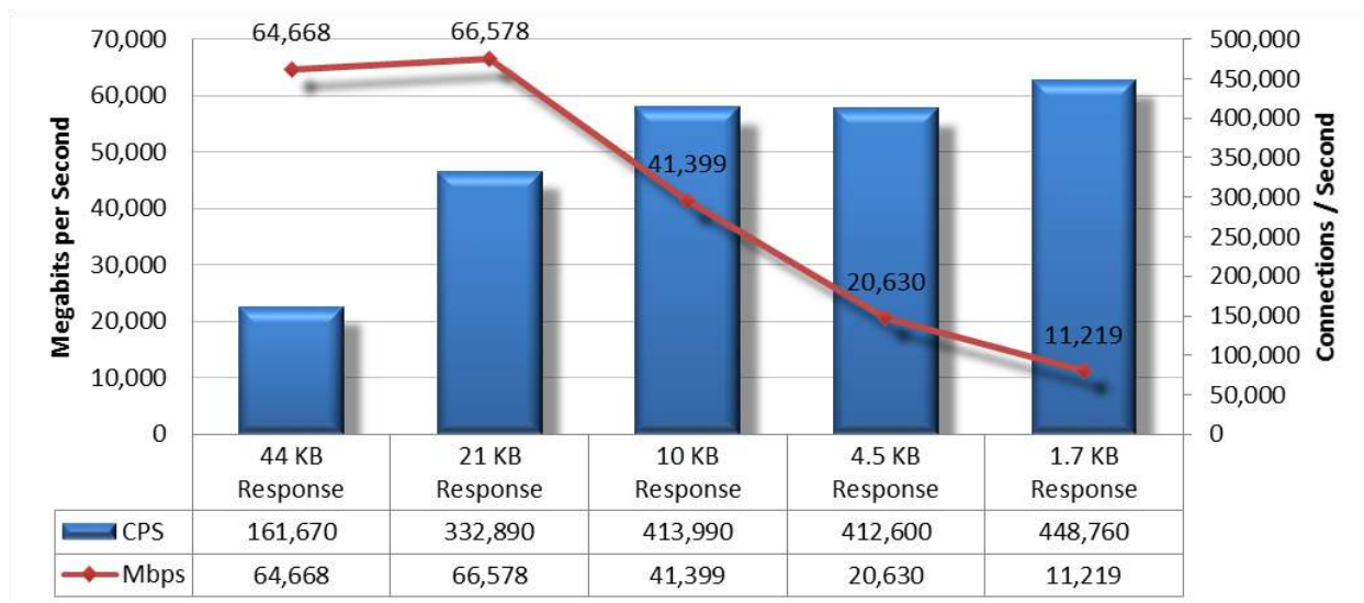
Figure 12 – HTTP Capacity with No Transaction Delays
